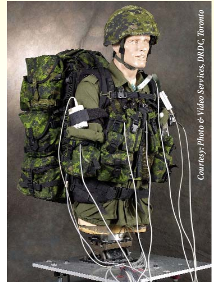
A Dynamic Load Carriage Simulator tests a Load Carriage System (webbing, load-bearing vests, patrol packs and rucksacks) – critical wear for soldiers.
