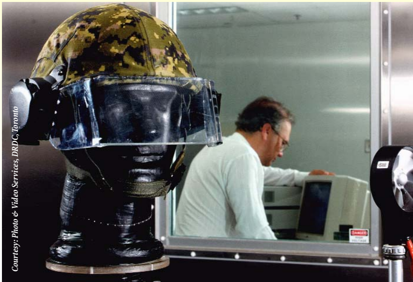
The Thermal Manikin Head, used to access the thermal insulation of head gear, measures heat loss from four separate zones.
